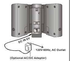
You may also purchase a "Universal" type AC/DC adapter which allows you to select the required output voltage and plug polarity, and normally includes multiple plug sizes to fit most brands of equipment. Always look for the "**UL**" listing mark when you purchase an adapter.
